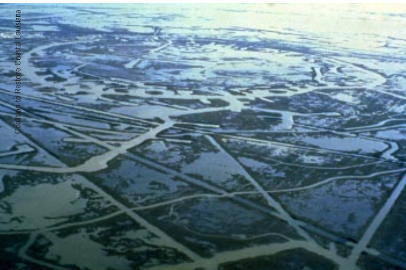
A century of navigation, mineral mining, and oil and gas activity have left the coast cross-cut by canals and spoil banks.
