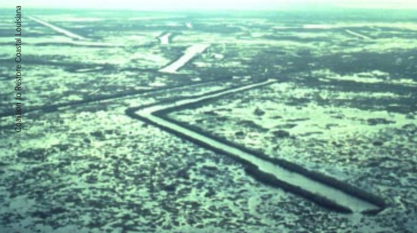
Canals and spoil banks create barriers to natural water flows and drainage.
